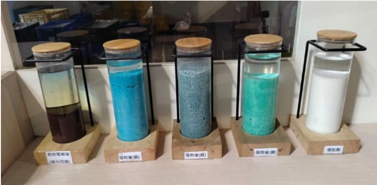
Waste liquid crystal glass transitioned to the adsorption material for wastewater treatment
