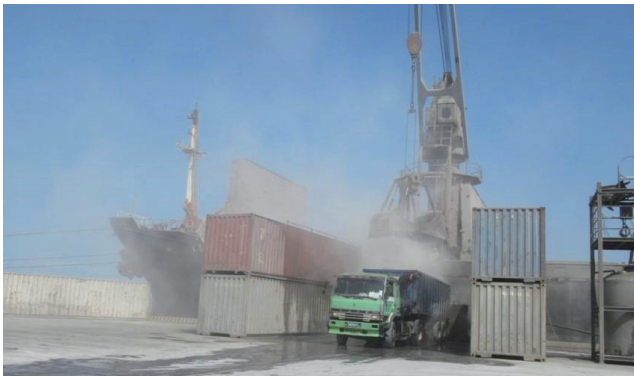
▲ During a discharge of cement clinker, visible particulate pollutants fill the air.
